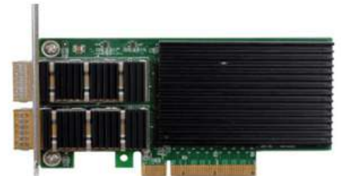
Netmon 160G2Q-XL Intel XL710 40Gbps Dual Port Fiber Optical Server Adapter Configurable Modes: • 1x40GbE + 1x40GbE • 1x40GbE + 4x10GbE • 4x10GbE + 4x10GbE
